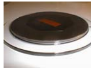
CNTEch standard mesa mask on NIST Format Glass Ring
